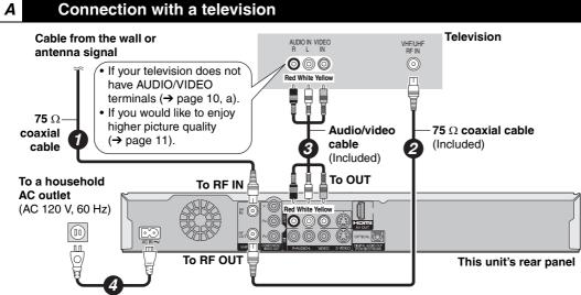
AC power supply cord (Included) Connect only after all other connections are complete.
