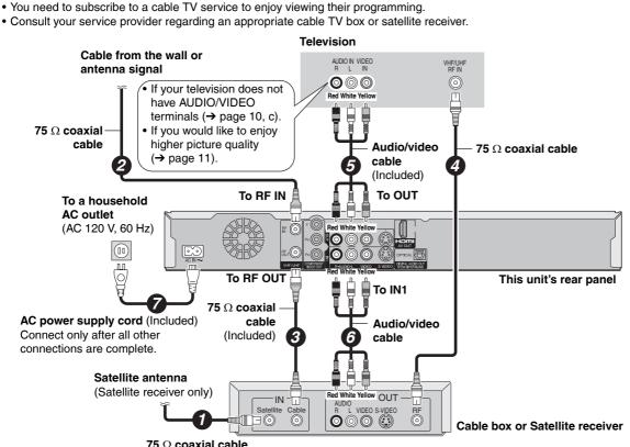
Connection with a television and a cable box or satellite receiver
